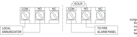
An uninsulated section of a single conductor should not be looped around the terminal and serve as two separate connections
